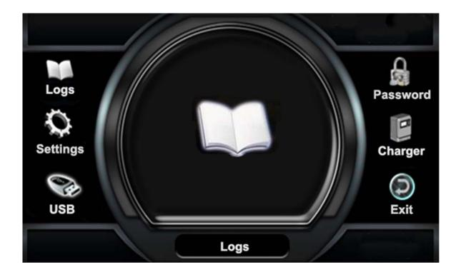
When the charger is idle, press and hold <ESC>, the Main Menu is then displayed. The main menu is automatically exited after 60 seconds of inactivity or can be exited voluntarily by pressing the <ESC> button.
