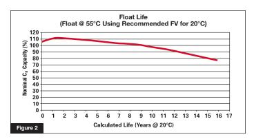
Battery life is reduced by 50% for every 10°C/18°F increase in temperature (see figure 3). Float voltage compensation reduces the charging current as battery temperature increases and partially negates the adverse effect of high temperature.
