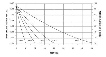
The maximum storage times before a refresh charge is required and recommended open circuit voltage audit intervals are:
