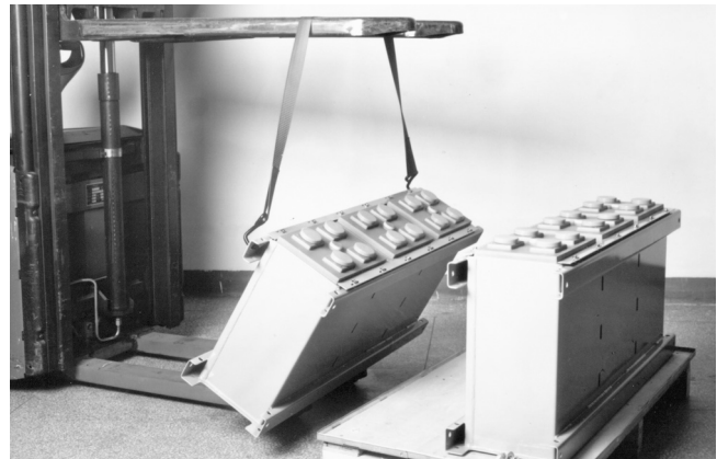
Figure 4: Lifting the module clear of the pallet
