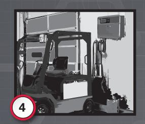
If battery is OFF, the charger automatically wakes battery and initiates charge.
