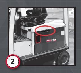
Connect charger cables to battery using the dedicated battery charging connector(s). Do not charge with cable that connects battery to equipment.
