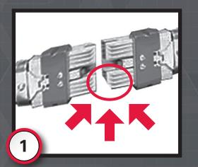
Prior to connecting, ensure cables have no damage and connectors are free of contamination.
