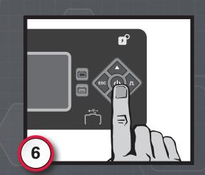
Press the charger's ON/OFF button before disconnecting battery from charger.
